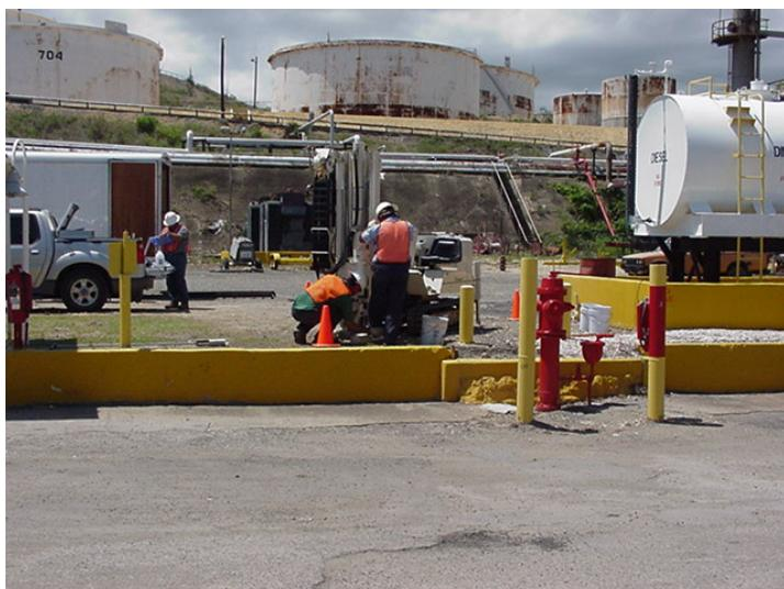
The 66DT unit is capable of obtaining water samples without the installation of monitoring wells or piezometers since it uses screened rods inserted in the ground to obtain water samples.
